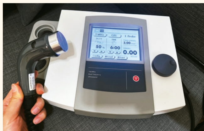
A typical therapeutic ultrasound machine, and its transducer probe
