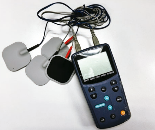
Typical appearance of a TENS machine: a small, battery-operated device that has leads connected to sticky pads (electrodes)
