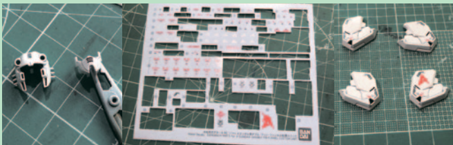
Line marking using enamel paint. Use cotton wool sticks to soak with lighter oil to remove color that are painted out-of-boundary
