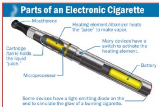
Fig 1 : Parts of an Electronic Cigarette Source: Wikipedia ( https://en.wikipedia.org/wiki/Construction_of_electronic_cigarettes )
